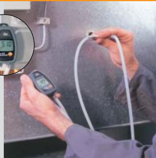
Measuring air flow with the Pitot tube
