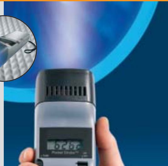
rpm measurement on a turbo ventilator
