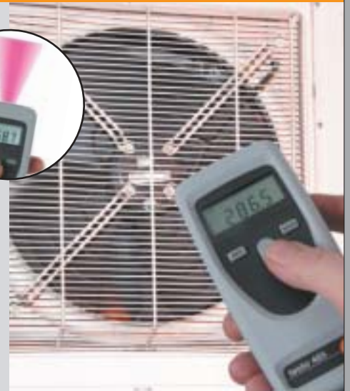
Rpm measurement on fans and ventilators
